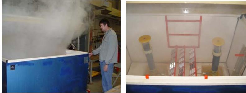
Figure 14. Two views of the salt fog chamber
