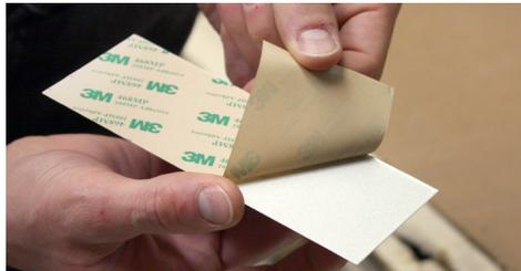
Make sure the area inside the frame is clean and free of debris. Place the label in the frame by positioning one edge of the label against the inside edge of the frame and then pressing the rest of the label firmly in place to insure a good bond.
