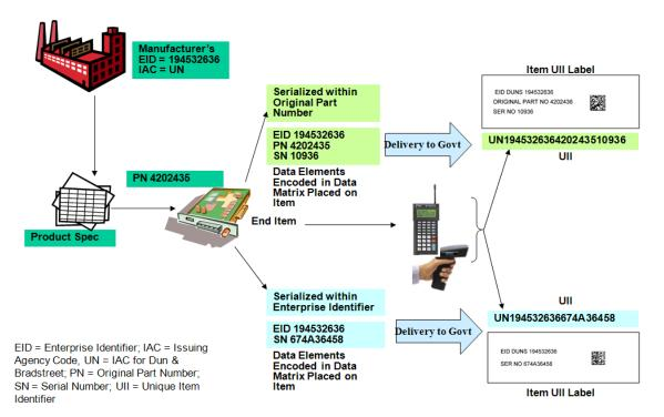
**Figure 3. UII Determination Process**
