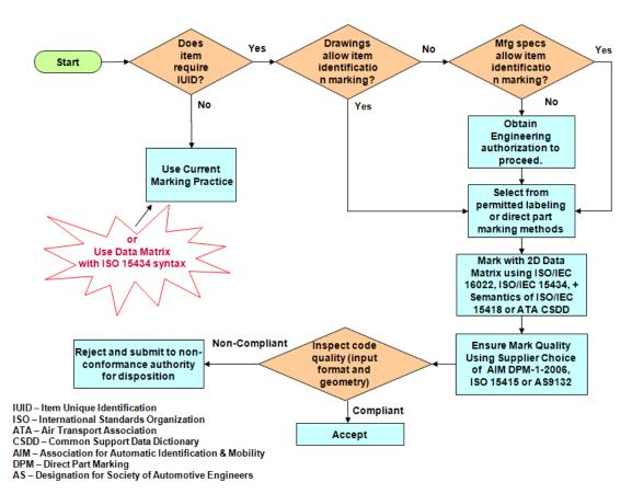
Figure 4. Supplier Considerations in Machine-Readable Information Part Marking
